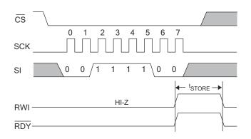
Figure 38. Software RECALL Cycle
