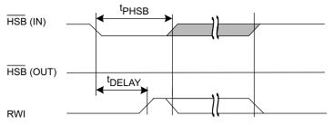
$\overline{\text{HSB}}$  pin is driven  $\underline{\text{HIGH}}$  to  $V_{CC}$  only by Internal 100 K $\Omega$  resistor,  $\overline{\text{HSB}}$  driver is disabled SRAM is disabled as long as HSB (IN) is driven LOW.
