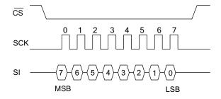
The two SPI modes are shown in Figure 4 and Figure 5. The status of clock when the bus master is in standby mode and not transferring data is:
