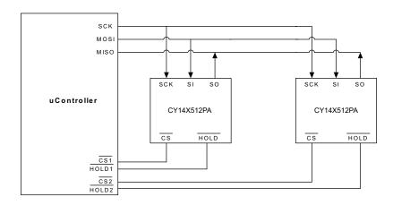
Figure 3. System Configuration Using SPI nvSRAM
