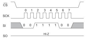
To issue this instruction, the device must be write enabled (WEN bit = '1'). The instruction is performed by transmitting the STORE opcode on the SI pin following the falling edge of CS.
