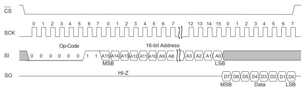
Figure 12. Burst Mode Read Instruction Timing
